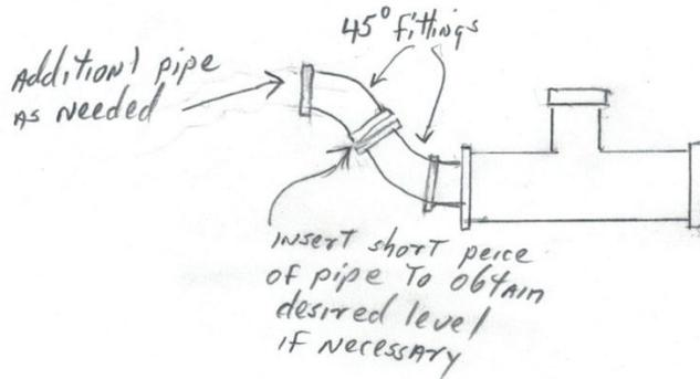
2. Add a piece of plastic to the down-stream side of the foam exit on the "T". This should extend an inch or more into the "T". This will help the bubbles escape through the foam exit and, by forcing the water to take a lower route, will help insure that the foam is not dumped back into the pond. For this piece you might use a small section of pipe, cut lengthwise to form a channel. Or use a piece of plastic cut from the side of a bucket or plastic container.
