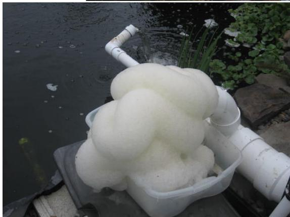
Please note the color of the foam. The whiter the foam, the cleaner your water. The darker foam is caused by very small suspended particles attaching to the foam. Your goal should be to have white foam. Eventually, as the DOC’s are removed, you should have very little or no foam.
